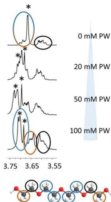
**Figure 3.** NMR resonance signals of 100 mM PEG200 in the presence of 0, 25, 50, and 100 mM PW (from top to bottom) and qualitative assignment of the protons of the main component of PEG200, that is, EO<sub>4</sub>, to the resonance signals. The stars indicate the change in intensity of the resonance signal stemming from the inner protons (blue circles) and the emergence of a doublet of PEG200, which represents PEG200 adsorbed on PW.
