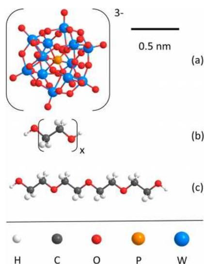
**Figure 1.** Optimized structures of (a)  $\alpha\text{-H}_3\text{PW}_{12}\text{O}_{40}$  (PW), (b) the  $\text{EO}_x$  oligomer repeating unit, and (c) the main component in PEG200, that is,  $\text{EO}_4$ . PW– $\text{EO}_x$  interactions were investigated as a function of its ratio,  $\text{EO}_x$  chain length and  $\text{EO}_x$  concentration. Polydisperse PEG chemicals (PEG200, PEG300, PEG400, and PEG20000) were used to cover a broad range of  $\text{EO}_x$  oligomer chain lengths.
