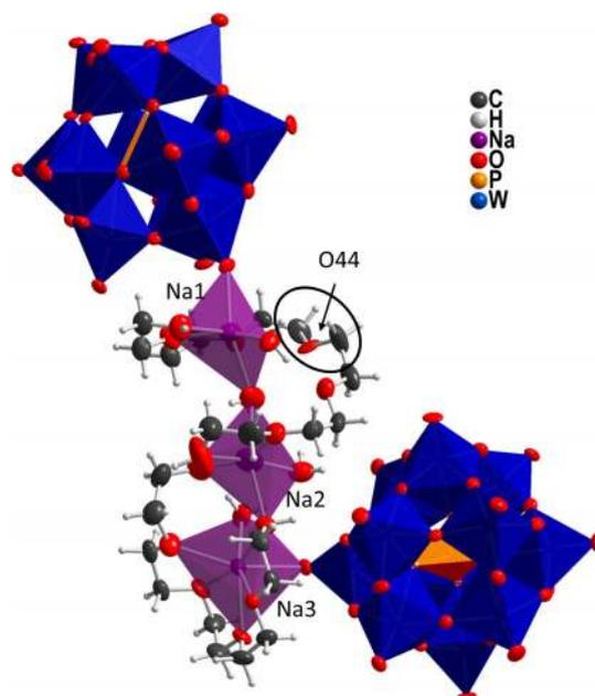
**Figure 6.** Representation of the coordination polyhedra of Na<sup>+</sup> (Na1: distorted octahedron, Na2: distorted octahedron, and Na3: distorted pentagonal bipyramid). The black circle indicates the disordered fragment of the EO<sub>6</sub> chain in the crystalline compound due to a long interatomic distance *d*(O44A–Na1) = 2.77 Å and *d*(O44B–Na1) = 3.25 Å, respectively. This fragment was refined with split positions; only the major contribution is shown here.
