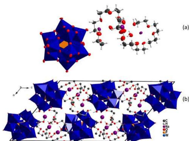
**Figure 5.** (a) Asymmetric unit of the structure model of C<sub>22</sub>H<sub>56</sub>Na<sub>3</sub>O<sub>57</sub>PW<sub>12</sub> represented with displacement ellipsoids (probability factor 70%). Split positions are not shown in this representation. (b) Packing of the elementary cell projected along [010]. For the sake of clarity, atoms are not displayed with displacement ellipsoids and hydrogen atoms connected to carbon are omitted.
