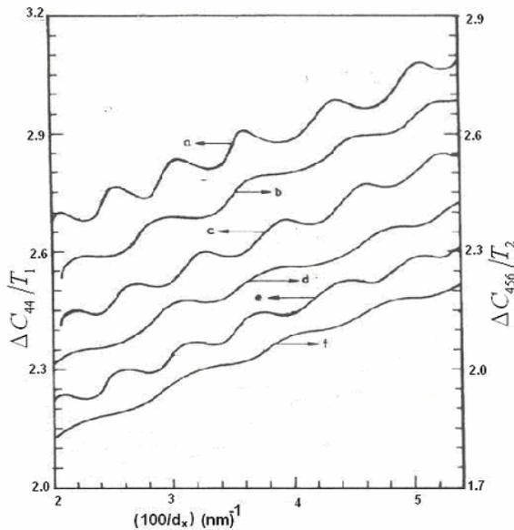
Figure 1. The curves e and f, d and c and b and a exhibit the plots of the normalized  $\Delta C_{44}$  and  $\Delta C_{456}$  as functions of inverse  $d_x$  for QWs, QWWs and QDs of CdGeAs<sub>2</sub> respectively.
