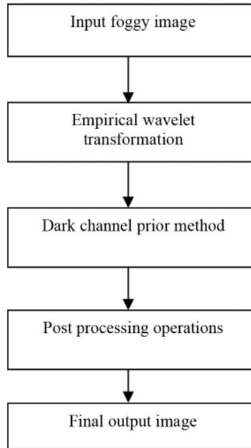
Fig. 1 Block diagram of proposed algorithm
