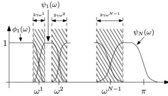
**Fig. 2** EWT boundary generation and filter construction
