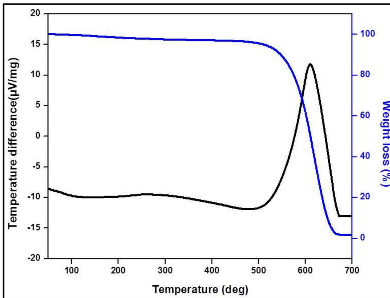
Fig. S7. Temperature programmed oxidation of CNFs after oxidation ( $\text{HNO}_3$ ) treatment. It clearly confirms on-set oxidation only at temperature  $> 800\text{K}$  indicating the stability of CNFs and resulting carbon showed graphitic character (Chen et al., 2009).
