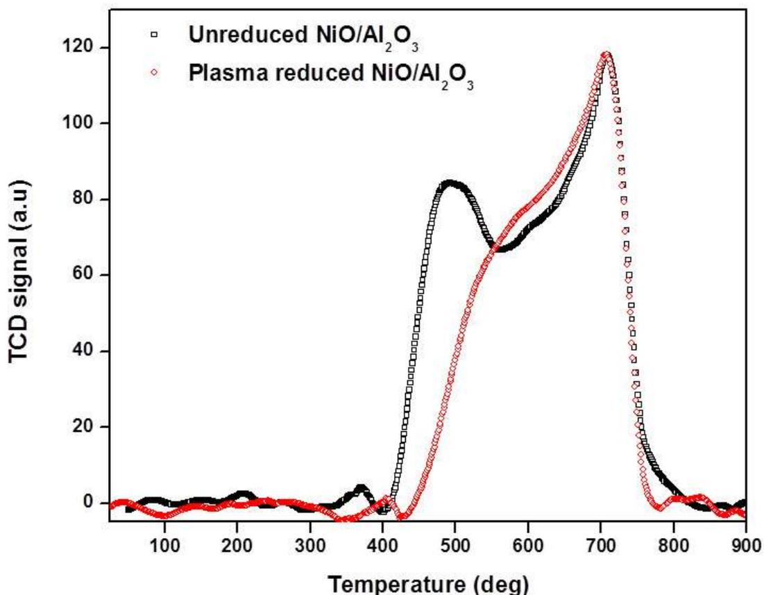
Fig. S2. TPR spectra of NiO/Al<sub>2</sub>O<sub>3</sub> catalyst (Black) , H<sub>2</sub> plasma-reduced NiO/Al<sub>2</sub>O<sub>3</sub>( Red).
