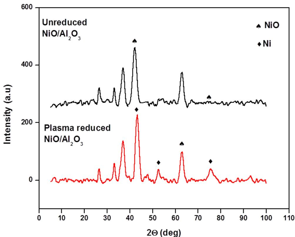
Fig. S1. XRD patterns of NiO/Al<sub>2</sub>O<sub>3</sub> catalyst a) no treatment, b) after H<sub>2</sub> plasma-reduction
